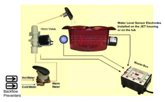
Fig. 1 Connection Diagram
