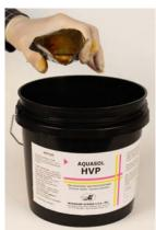
After pouring the diazo into the emulsion, check the inside of the bag for any remaining diazo. You can add a small amount of water to dissolve any remaining diazo in the bag and add to the emulsion.
