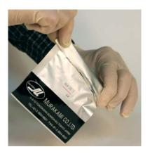
Use a side to side motion for about 15 seconds to melt all of the emulsion in the bag. Keep folded top well sealed. Tilt bag to dissolve all diazo in bag.
