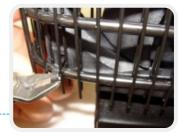
Cut the four black plastic strips holding the fan to the condenser
