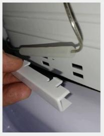
Remove the plastic element fixing the thermostat from the evaporator
