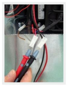
Disconnect wires of fan from + and F of the ECU and check if there is continuity. If not replace fan.
