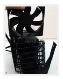
Remove the fan from condenser and reverse the procedure to install the new one
