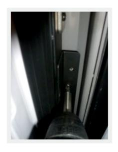
◆ Unscrew the 4 screws of the bracket
