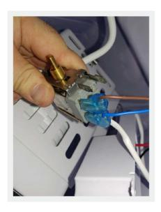
◆ Detach the wires from the thermostat, pull out the thermostat and reverse the procedure to install the new thermostat
