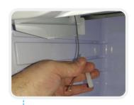
Remove the rubber cap from the sensor of the thermostat
