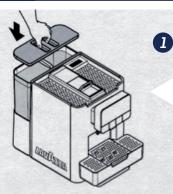
At first use, remove the tank from back, rinse and then fill with water. Replace the tank ensuring it is locked into place and place the lid on top.
