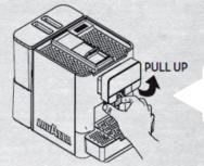
Insert Lavazza BLUE capsule into top of machine and close the hatch by pulling forward.
