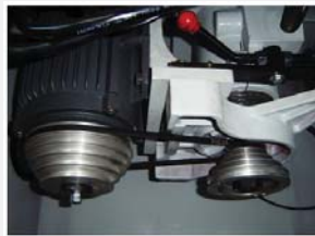
Powerful 7.5 HP motor with 5 spindle speeds
