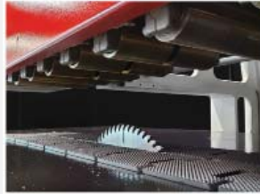
11 hold down rolls and bottom mounted saw blade
