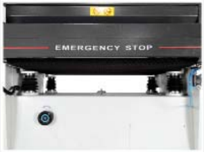
Four table elevation jack screws and emergency stop bump bar
