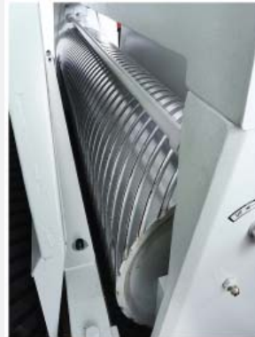
Steel contact drum with micro adjustment
