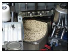
**GLUE POT**The 1.2 kg Teflon-coated glue pot is designed for EVA hot-melt glue. The glue is applied by a roller and the glue amount is adjustable
