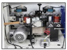
**GUILLOTINE SHEARS**Coiled material up to 3 mm in thickness can be trimmed by the guillotine shears
