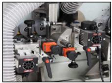
**FLUSH AND RADIUM TRIMMING UNIT**The adjustment of the settings from flush to beveled finish for thin edges, as well as radius trimming for thicker edges, is quick and easy.
