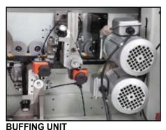
The buffing unit leaves a super finish on ABS and PVC edging, and removes any discoloration on the edges, which is especially noticeable when working with dark edge material
