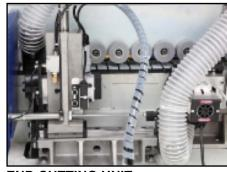
**END CUTTING UNIT**Mounted on high-precision linear bearings, which ensure perfect cutting results for years to come. The high frequency 12,000 RPM motor meets any challenge regardless of edge type and thickness
