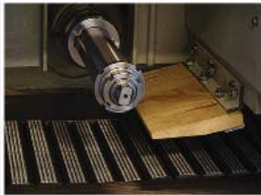
Precision cast iron chain, nickel chrome arbor with removable saw sleeve
