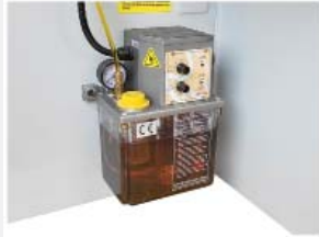
Automatic lubrication unit for chain and track assembly
