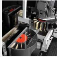
Side brush sanding units with independent adjustment
