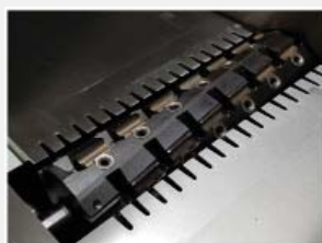
Spiral insert knife cutterhead with 30 x 12 x 1.5 mm two-sided insert knives
