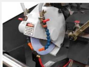
Precision dresser assembly with straight and radial diamond dresser mounted above the wheel for easy access
