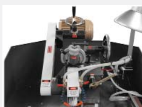
Convenient wheel angle adjustment (side clearance). Motorized setting optional
