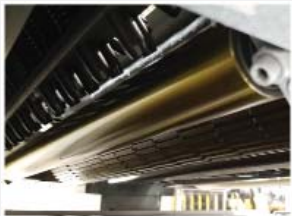
Section chip breaker, sectional infeed roll before top planer head
