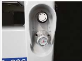
Variable feed speed and micro table height adjustment controls
