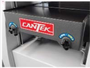
Adjustable infeed and outfeed bed rolls
