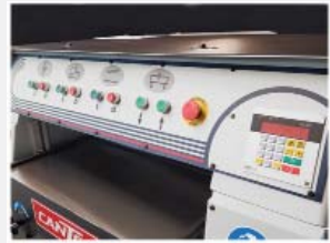
Operator controls with digital thickness control unit
