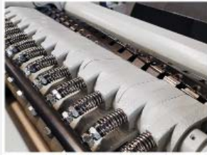
Cast iron planer assembly with sectional chipbreakers and spiral insert knife cutterhead
