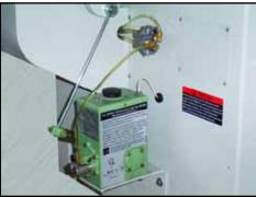
**MECHANICAL CHAIN LUBRICATION** Lubricant flow rate can be adjusted automatically with the caterpillar chain feed speed variation. When lubrication runs out the chain stops automatically preventing damage to the machine.
