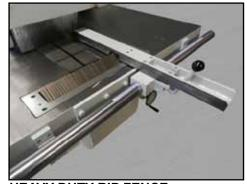
**HEAVY DUTY RIP FENCE** Quick setting rip fence runs on round cylindrical guide. Fence is notched to pass over and under the table and top kickback fingers for faster change over.
