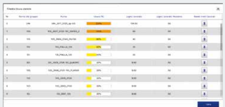
Display of the tools wear status.
