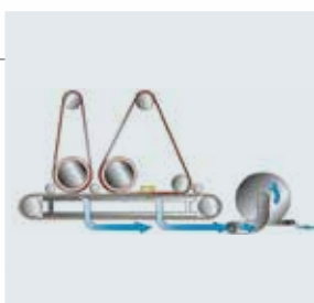
Vacuum table no slipping of the work piece.
