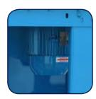
Dedicated fan motor ensures optimum air flow for proper temperature control. Safety shutdown feature is enabled when cooling fan power is interrupted.
