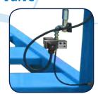
This automatic drain valve removes condensate from the moisture separator trap at the discharge of the after-cooler
