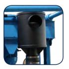
Heavy duty, dry-type air intake filter enhances air quality before it touches the main components of the machine. This lengthens the lifetime of the machine. The element is conveniently
