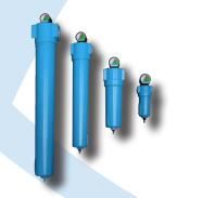
FHO inline filtration comes standard with differential pressure gauges and are protected with an interior and exterior powder coating finish. They hold a replaceable filter that can be quickly and inexpensively maintained. All housings come standard with internal float style drain valves.
