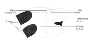
Charging Port – This is used to recharge your Spryng device using a USB charging cable Velcros – These are used to fasten your Spryng devices
