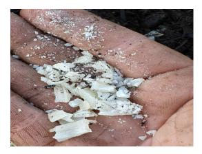
The inspection on day 8 revealed that the product disintegrated and we could therefore not differentiate between the product and the rest of the windrow's material. The product was also too small to detect due to our process of turning the windrow with a self-propelled turner.
