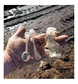
Product were placed back into the windrow and operation went on as normal. Windrow was maintained at temperatures between 65 and 70 degrees with a moisture content of 45 - 48%.
