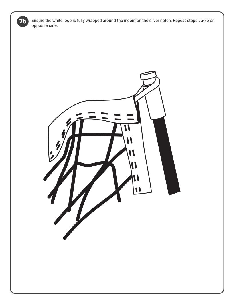
**FOR FRONT OF NET**: Hook the white loop located at the front top corner of the **Net** to the silver notch located on the **Upper Pole**.
