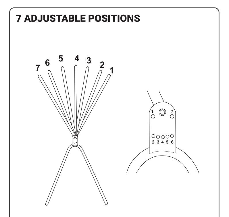
Adjust the pin position on both **Swivel Hinges** to create everything from groundball to flyball positions.
