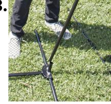
3. Insert one lower (thicker) bar into post at base leg. Repeat for other side.
