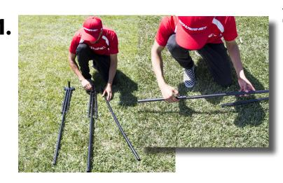
1. Attach middle bar into both ends of the base legs.
