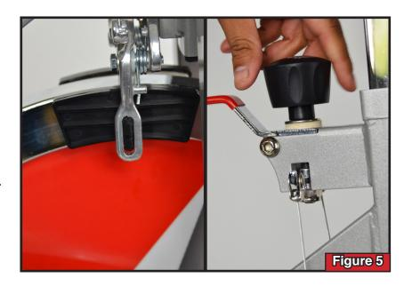
**Note:** Inspect the brake pads for wear on the cycle. Replace the felt brake pads if they are visibly worn.
