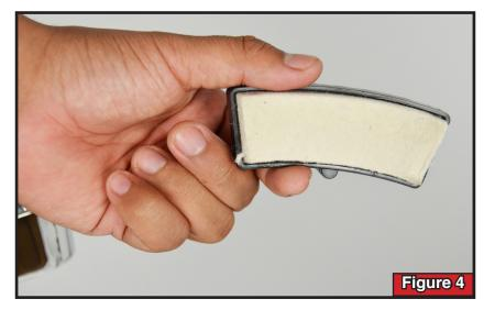
Step Five: After the lubricant has been applied, slide the brake pad between the flywheel and its metal bracket. Tighten the brake tensioner to your desired setting for next use (see Figure 5).
