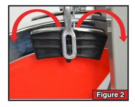
**Step Three:** When the brake pad is detached, inspect it for any dirt and debris. Use a brush or any other abrasive material to scrub the brake pad. (see **Figure 3**).
