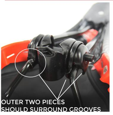
**STEP 3:** Now place the final groove (4) pieces outside the bike's seat brace and lock together with the nuts (3). Make sure to screw these pieces together tightly for a secure fit. You have successfully put your seat's clamp back together! Revisit page 1 to place the seat on the bike's stem.
