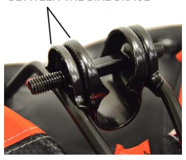
**STEP 2:** Take the ridges (5) and place the teeth alongside the clamp (1). Notice that they have grooves that will lock onto the bike's seat brace. (see left photo) These pieces should sit between the bike's braces. For a better photo, view step 2 continued.
