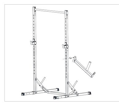
Insert the attachment into the Upright Frame. Turn as arrow showed to tighten.
