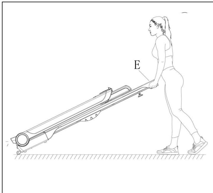
To transport, hold the treadmill at Position E and tilt until the transportation wheels can move smoothly.
