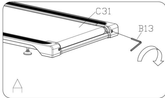
If the **Running Belt (No. C31)** moves to the left, turn the left adjusting bolt  $\frac{1}{4}$  turn *clockwise*, then turn the right adjusting bolt  $\frac{1}{4}$  turn *counter-clockwise*. If the **Running Belt (No. C31)** does not move, repeat this step until it centers. Refer to Figure B.
