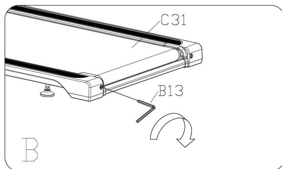
Over time the **Running Belt (No. C31)** will loosen. To tighten the **Running Belt (No. C31)** turn the **Left & Right** adjusting bolts one full turn *clockwise*, check the tension of the **Running Belt (No. C31)**. Continue this process until **Running Belt (No. C31)** is at the correct tension. Make sure to adjust both sides equally to ensure correct belt alignment. Refer to Figure C.
