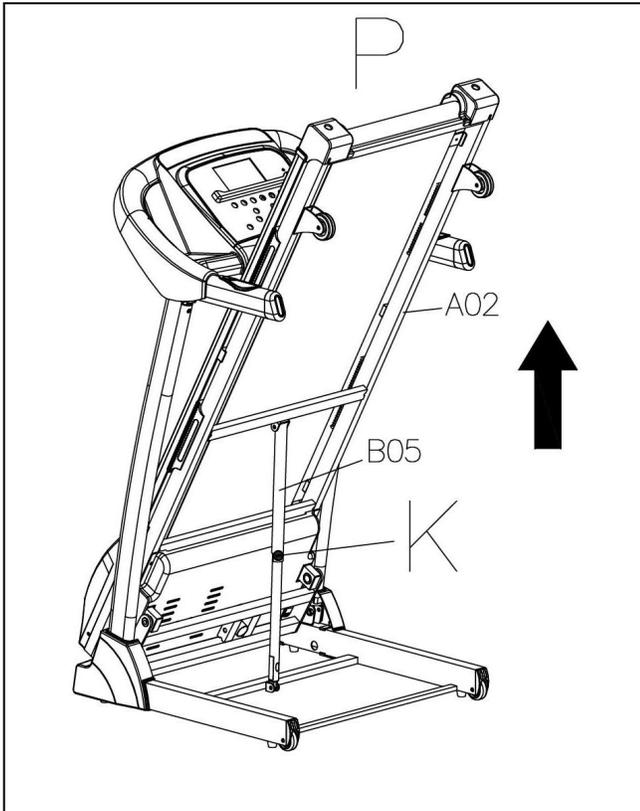
**NOTE:** Please make sure the incline is at ZERO when folding and unfolding.
