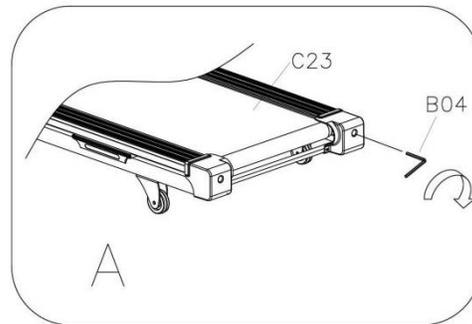
If the **Running Belt (No. C23)** moves to the left, turn the adjusting bolts  $\frac{1}{4}$  turn *clockwise*, then turn the right adjustment bolt  $\frac{1}{4}$  turn *counter-clockwise*. If the **Running Belt (No. C23)** does not move, repeat this step until it centers. Refer to Figure B.
