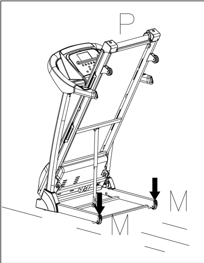
Before attempting to move the treadmill, make sure that it has been properly folded. Unplug the power cord.
