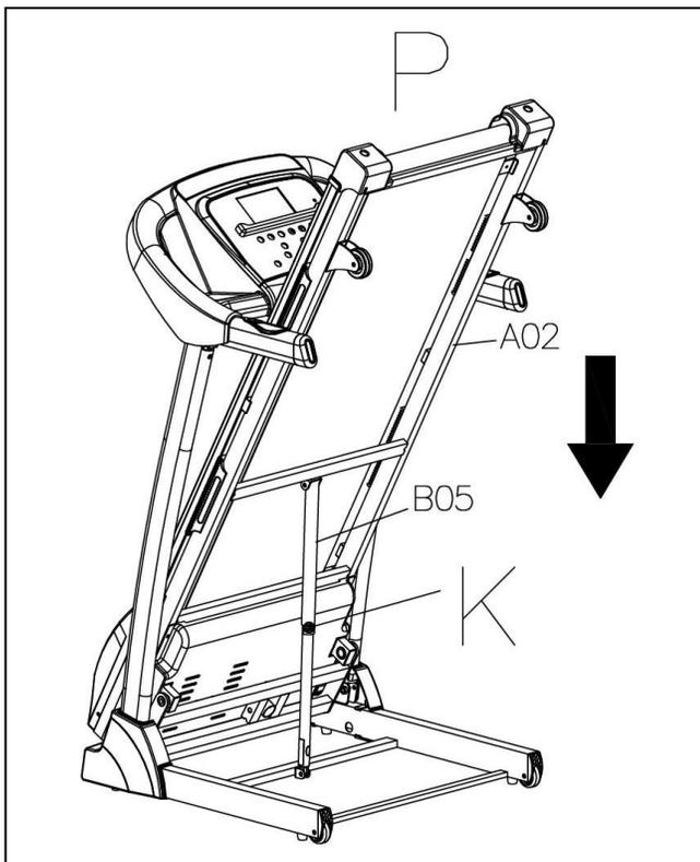
Before lowering the **Main Frame (No. A02)**, ensure that the space directly underneath it is clear of any objects.
