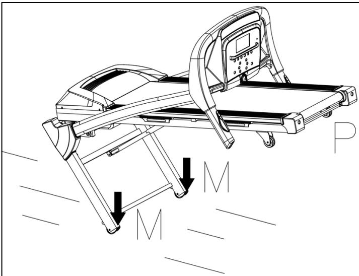
To transport, hold the treadmill at position "P" and tilt until the transportation wheel's "M" are able to move on the ground.
