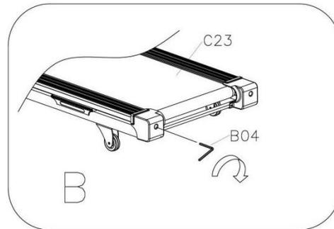
Over time, the **Running Belt (No. C23)** will loosen. To tighten the **Running Belt (No. C23)**, turn the Left & Right side adjustment bolts one full turn *clockwise*, check the tension of the **Running Belt (No. C23)**. Continue this process until **Running Belt (No. C23)** is at the correct tension. Make sure to adjust both sides equally to ensure correct belt alignment. Refer to Figure C.
