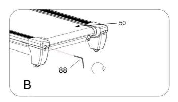
3. Over time, the Running Belt (No. 50) will loosen. To tighten the Running Belt (No. 50), turn both the left & right sides adjusting bolts one full turn *clockwise*. Check the tension of the Running Belt (No. 50). Continue this process until Running Belt (No. 50) is at the correct tension. Make sure to adjust both sides equally to ensure even alignment. Refer to image C.
