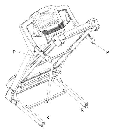
To transport, hold the treadmill from position "P" and tilt until the wheel's "K" are able to move on the ground.
