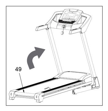
**NOTE:** Please make sure the incline is at ZERO when folding and unfolding.
