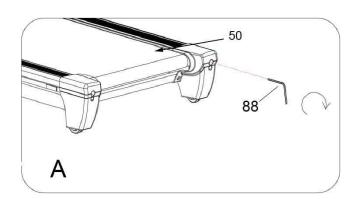
2. If the Running Belt (No. 50) drifts to the left, turn the left adjusting bolt ¼ turn *clockwise*, then turn the right adjusting bolt ¼ turn *counter-clockwise*. If the Running Belt (No. 50) does not move, repeat this step until it centers. Refer to image B.
