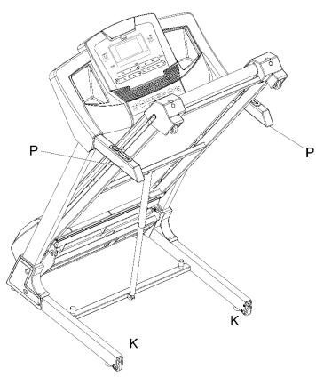
Before attempting to move the treadmill, make sure that it has been properly folded. Then, unplug the power cord.
