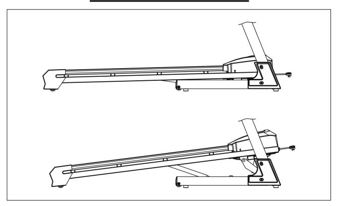
Console Keys and + - INCLINE Handrail Keys are used to control the incline level. Increase or decrease the incline level by pressing the incline buttons once per level or holding an incline key down to skip through to the desired level.
