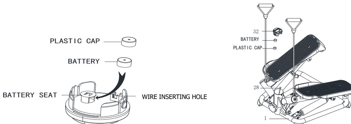
1. Remove **Computer (No. 32)** from **Main Frame (No. 1)** and disconnect the link wire of **Sensor (No. 28)** from the **Computer (No. 32)**.
