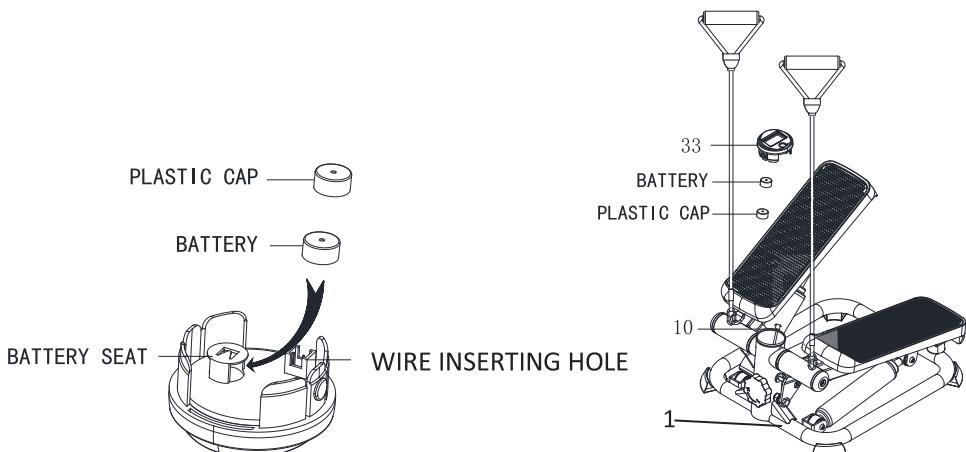
1. Remove **Computer (No. 33)** from **Main Frame (No. 1)** and disconnect the link wire of **Sensor (No. 10)** from the **Computer (No. 33)**.
