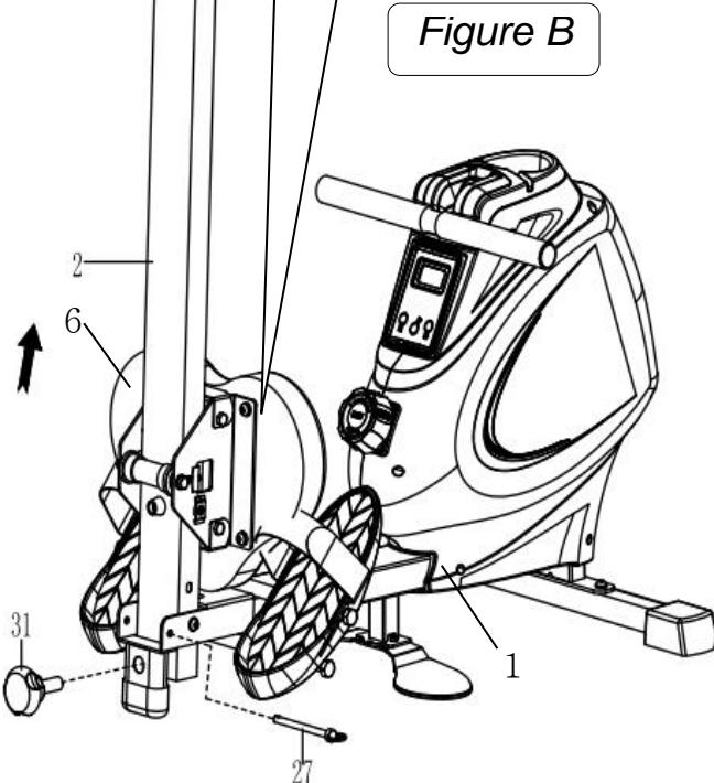
When not in use, you can save space by folding the **Sliding Rail (No. 2)**.
