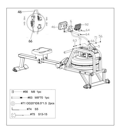
Remove 4 Screws (No. 64) from the Meter (No. 46) using Spanner (No. 75).
