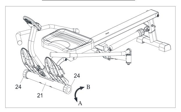
Before using, check the balance of the product to ensure it is safe for use. Put the product on a flat, even surface. If the product is slightly uneven, rotate the **End Caps** (No. 24) on the **Front Stabilizer** (No. 21) to compensate for the uneven ground.
