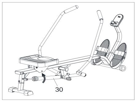
**NOTE:** Please do not adjust the resistance of the **Hydraulic Cylinder (No. 30)** during operation to avoid injury and damage to the rowing machine.
