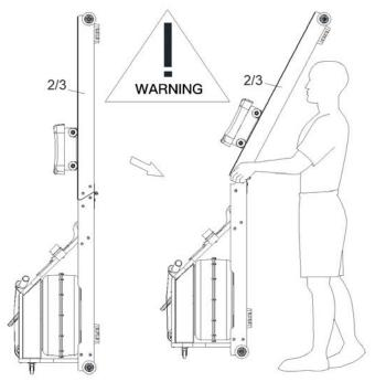
**WARNING!** Do not stand the rowing boat or lift the rail without folding and moving the rowing boat to prevent the rail or rowing boat from falling down and hurting people!
