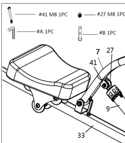
**Caution:** The **Hydraulic Cylinder (No. 9)** can generate excessive heat after long periods of use, making it unsafe to touch. Allow the **Hydraulic Cylinder (No. 9)** to cool before moving the rowing machine.
