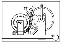
6. If you still hear noises after you did STEP 4 and STEP 5, please remove the **Left & Right Belt Covers (No. 105L & No. 105R)**. Loosen the **Hex Thin Nut (No. 87)** for the **Flywheel (No. 94)** about a half of a rotation. See the following diagram below.
