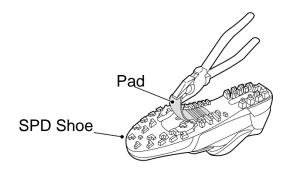
2. Remove the sockliner and install the cleat set according to the following illustration. Then, secure the cleat tightly with the bolt using Allen Wrench.
