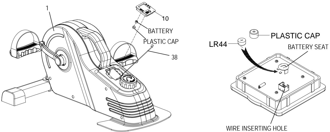
Remove the **Meter (No. 10)** from **Main Frame (No. 1)**. Then disconnect the link wire of **Inductor (No. 38)** with the **Meter (No. 10)**.
