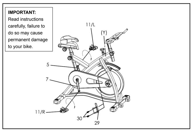
Connect Pedals L/R (No. 11) onto the Left and Right Crank Arms (No. 5 and No. 7). (Before you begin, immobilize the crank arms by turning the tension knob all the way to the right).
