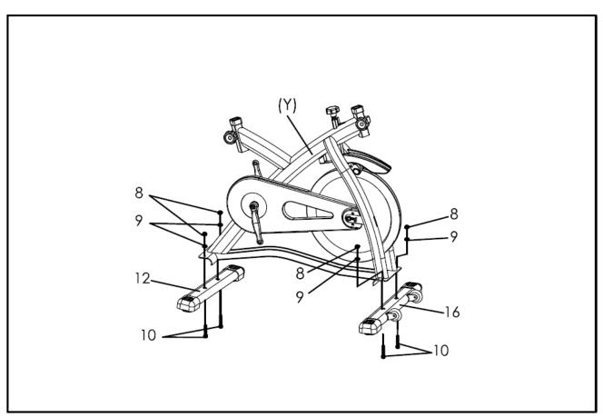
Attach the Front Stabilizer (No. 16) and the Rear Stabilizer (No. 12) to the Main Frame (Y) using 4 Bolts (No. 10), 4 Washers (No. 9) and 4 Nuts (No. 8). Tighten and secure using spanner wrench.
