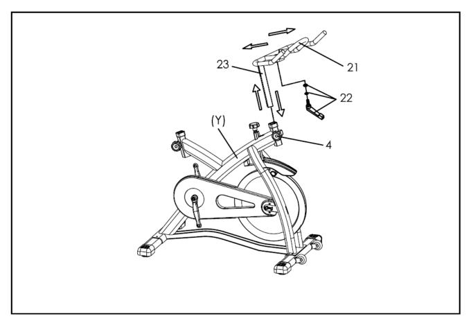
Loosen **Adjustment Knob (No. 4)** on main frame handlebar tube to remove protection cap, then slide the **Handlebar Post (No. 23)** into the handlebar tube of the Main Frame (Y).
