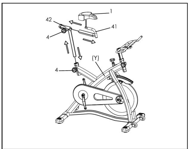
Insert the **Seat Post (No. 42)** into the seat tube located on the Main Frame (Y).
