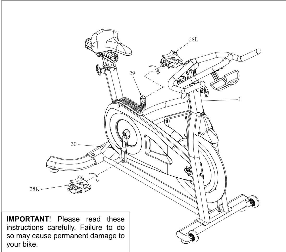
Connect **Pedals L/R (No. 28)** onto the **Left and Right Crank Arms (No. 29 & 30)**. Before you begin, immobilize the crank arms by turning the **Resistance Knob (No. 57)** all the way to the right.
