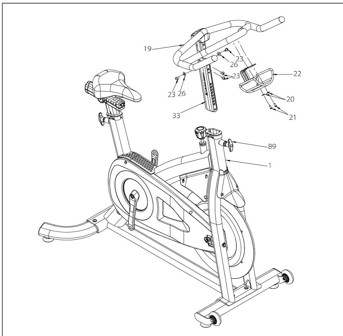
Insert the **Handlebar Post (No. 33)** into the front tube of the **Main Frame (No. 1)**. Use the **Handlebar Adjustment Knob (No. 89)** to adjust the handlebar to the desired height and secure the handlebar in position.
