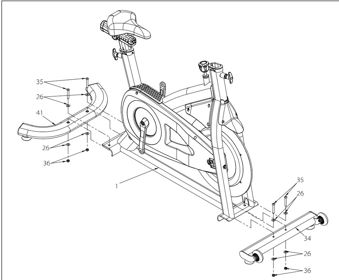
Attach the **Front and Rear Stabilizers (No. 34 & No. 41)** to the **Main Frame (No. 1)** using **4 Hex Screws (No. 35)**, **8 Flat Washers (No. 26)** and **4 Nylon Nuts (No. 36)**. Tighten and secure using **Hex Wrench (No. C)** and **Combination Wrench (No. D)**.
