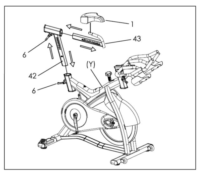
Insert the Seat Post (No. 42) into the seat tube located on the Main Frame (Y).
