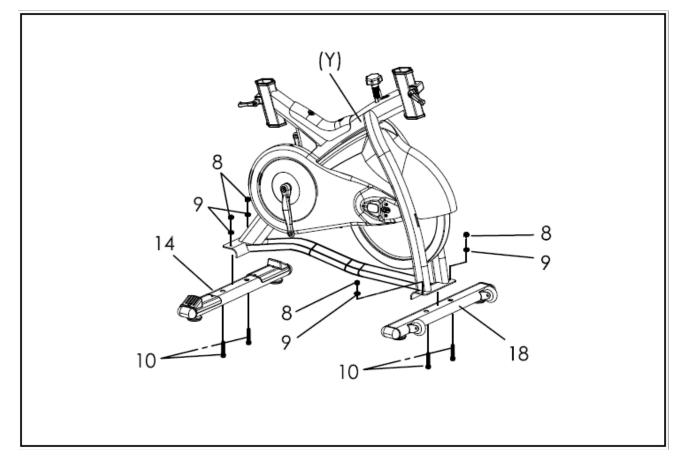
Attach the **Front Stabilizer (No. 18)** and the **Rear Stabilizer (No. 14)** to the Main Frame (Y) using 4 **Bolts (No. 10)**, 4 **Washers (No. 9)** and 4 **Nuts (No. 8)**. Tighten and secure using spanner wrench.
