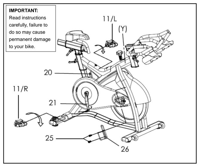
Connect **Pedals (No. 11)** onto the **Left** and **Right Crank Arms (No. 20 and No. 21)**. (Before you begin, immobilize the crank arms by turning the tension control knob all the way to the right).
