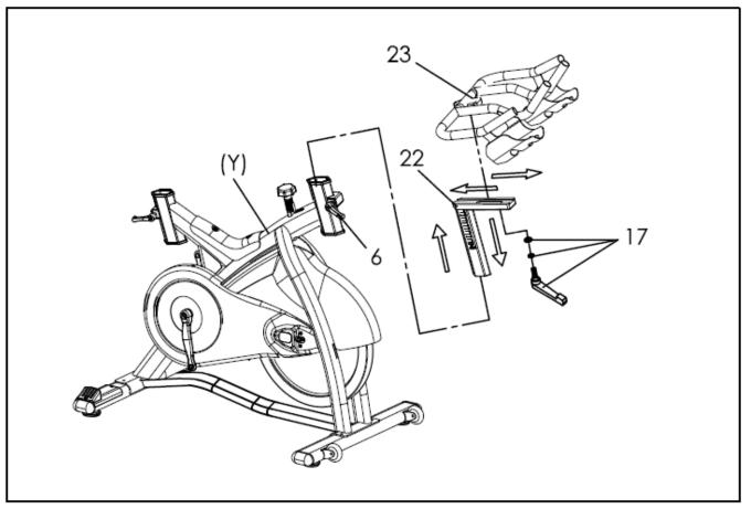
Loosen L-Shaped Knob 1 (No. 6) on main frame handlebar tube to remove insert protect cap, then insert the Handlebar Post (No. 22) into the handlebar tube of the Main Frame (Y). Adjust Handlebar Post (No. 22) to the desired height. Tighten the L-Shaped Knob 1 (No. 6) to secure the Handlebar Post (No. 22) into position.
