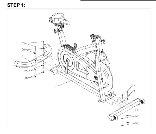
Attach the Front and Rear Stabilizers (No. 34 & No. 41) to the Main Frame (No. 1) using 4 Hex Screws (No. 35), 8 Flat Washers (No. 26) and 4 Nylon Nuts (No. 36). Tighten and secure using Hex Wrench (No. C) and Combination Wrench (No. D).
