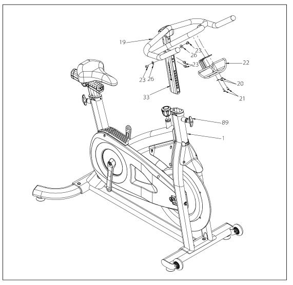
Insert the Handlebar Post (No. 33) into the front tube of the Main Frame (No. 1). Use the Handlebar Adjustment Knob (No. 89) to adjust the handlebar to the desired height and secure the handlebar in position.
