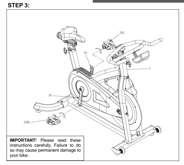
Connect Pedals L/R (No. 28) onto the Left and Right Crank Arms (No. 29 & 30). Before you begin, immobilize the crank arms by turning the Resistance Knob (No. 57) all the way to the right.
