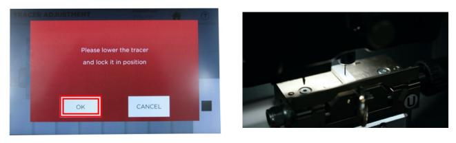
Loosen the tracer knob, lower the **TRACER** until it lands on the setup template, **tighten** the **KNOB**. PRESS OK
