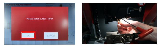
Install the CUTTER V037. PRESS OK
