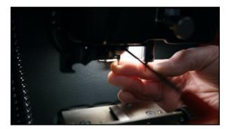
Install the T00 Calibration **TRACER** from the tool kit into the cutter spindle. Tighten the set screw and **CLOSE THE SHIELD**. **PRESS OK**
