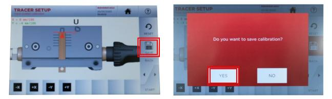
Write down the X & Y values and **PRESS THE SAVE BUTTON**. **PRESS YES** to save the results.
