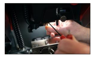
REMOVE the V037 CUTTER. PRESS OK
