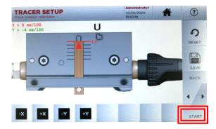
Insert setup template into jaw PRESS START.
