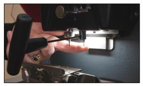
Remove tracer using 2.5mm allen tool, then select OK
