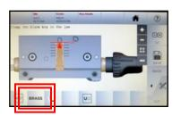
To change the material type, simply touch the BRASS icon on the screen until you reach the desired material; **BRASS, STEEL, NiSi** (Nickel Silver) or **ALU** (aluminum)
