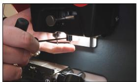
Install new tracer until it stops and tighten down set screw with 2.5mm allen tool You must perform the tracer setup, tracer adjustment and jaw calibration
