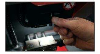
Loosen the tracer knob, lower the TRACER and tighten the knob. PRESS OK
