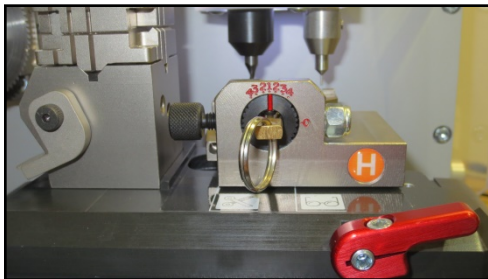
Fig. 1 Jaw in cutting position with template in 1 position
