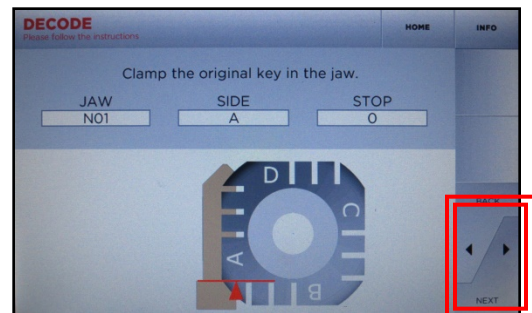
Insert key on jaw, then remove tip stop . Close shield and select NEXT
