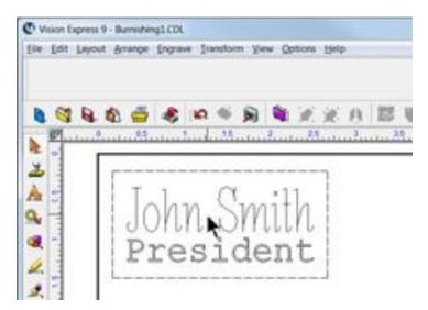
After clicking in the center of the plate, all fields are merged and multiple plate objects will be created based on the number of text variables selected.
