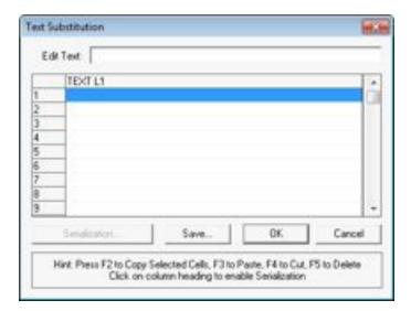
The text for the keys can be manually entered by typing in the text and pressing Enter on your computer keyboard. Once the text has been entered for all of the keys, select OK.
