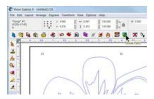
Next, we will need to create a path. The Vision 9 software has an intelligent path tool that will automatically detect portions of the graphic that are within outside vector lines and will create a hatch fill with the center portions left as unfilled. Press the F3 button on the computer keyboard to select all items, then select the Make Path icon.
