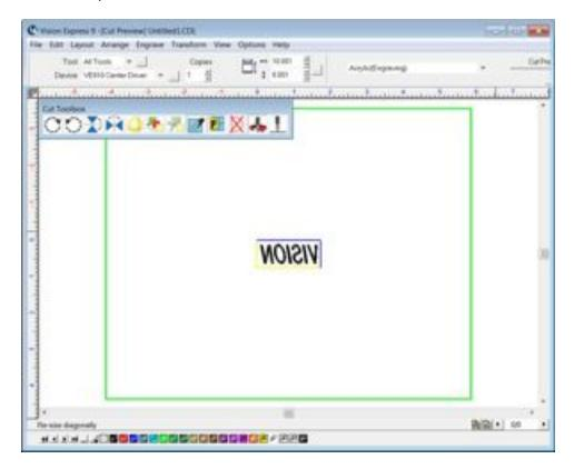
Select Engrave from the Cut Toolbox, then press the Start button on the engraver to begin engraving the job. You may want to perform a dry run before engraving to check for setup errors.
