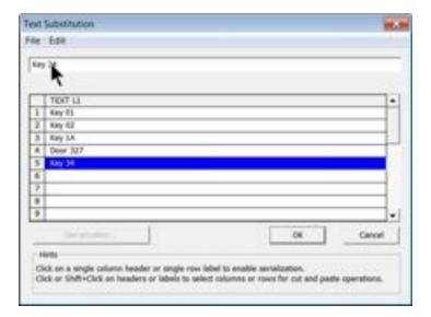
If the keys are to be automatically serialized, there is no need to manually enter the text. From the Text Substitution screen, click the text column header as shown. All of the blank fields will be selected and turn blue, then click on Serialization.
