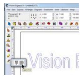
As with the previous example, the hatch fill is applied. Adjust the Tool width, Tool angle, Tool style and color as desired, then select Close. The file is ready to be sent to the engraver.
