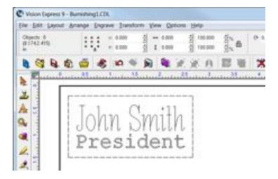
In this example, a text file was created in order to copy and paste the variables into the Vision software. Highlight the text and select copy from the edit menu (or right click and select copy). Note that in this example, the two variables are entered as subsequent lines in the text file and that there may be difficulties when importing from other file formats. A simple text file created in Windows Notepad is suggested.
