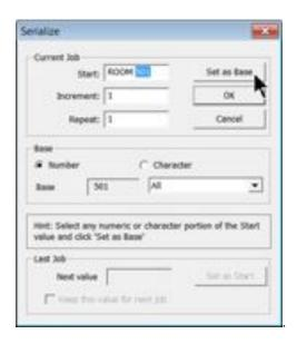
The serialized text will be shown in the Text Substitution window. If there is an error, select Serialization and re-enter the information, then select OK.
