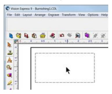
Enter any text in the format you wish to use. In this example, two lines of text are entered as variables (it does not matter what you type. The text entered is only for formatting and will be replaced with the text imported from the .txt file).
