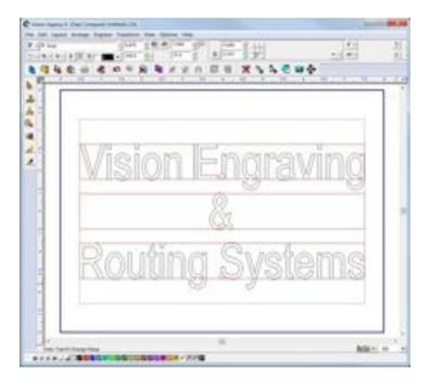
Before filling text, the user must first select the text with the Select Tools icon. Click on the Select Tools icon and select the text to apply the hatch fill to.
