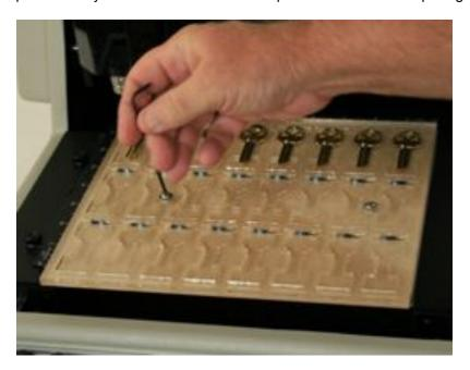
Once the keys have been installed in the fixture, send the file to the Engrave-IT Pro by first selecting the Engrave icon from the left toolbar.
