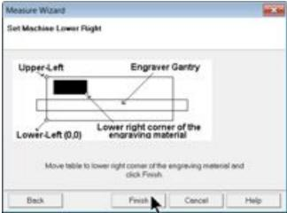
The dimensions of the plate size shown in the Plate Size window will now reflect the engraving area you have defined on the machine. The Home Position of the machine has also been set to the upper left corner of this area.
