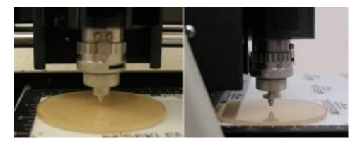
Select the Engrave icon from the left side toolbar. Double check to make sure that the Device is set to the VE810 Center Driver (on the top toolbar). Choose your material from the Material Setting drop down list on the top toolbar.
