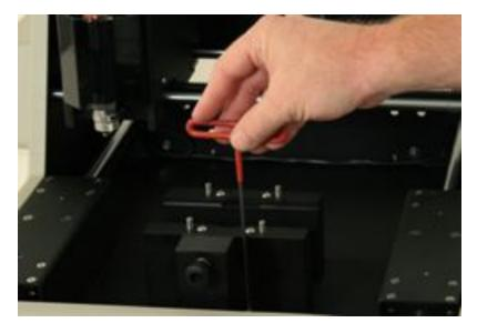
Slide the acrylic cylinder fixture onto the vise pins on the top of the vise. Install the cylinders into the fixture and tighten the handle on the vise to lock the cylinders securely.
