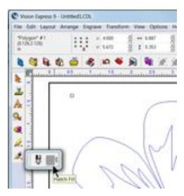
The hatch fill will be applied. Adjust the tool options as desired and select Close from the toolbar menu. The file is ready to be sent to the engraver.
