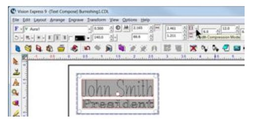
Change the settings to Always compress or expand text to fit width, Method: Width compress/expand, and Apply to: Each Line Individually. Deselect Word Wrap, then select OK.
