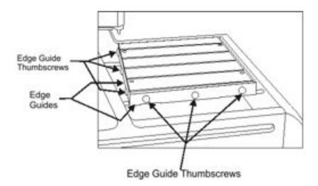
To adjust the edge guides, loosen the edge guide thumbscrews and raise them above the surface of the T-slot table. Place the material on the table, then loosen the edge guide thumbscrews and lower the edge guides until they are even with (or just below) the material surface. Tighten the edge guide thumbscrews. This process should be repeated any time materials of different thicknesses are to be engraved.
