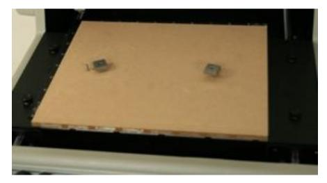
Turn the fixture back over and slide the fixture on the engraving table. Tighten the T-slot screws as shown below. To load the keys, insert the top of the key against the top of the key opening and then press the key into the slot. This is the simple and fast method of putting the keys in the holder.
