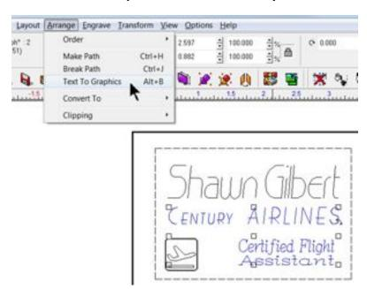
The two text fields are now non-editable graphics and will not be replaced when importing a text file with variable text. Next, copy the list of text variables from a Notepad text file and select Paste Clipboard Into Plate, then click in the middle of the Plate Object.
