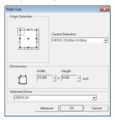
A single Plate Object will be created (from the top toolbar menu - Layout  $\longrightarrow$  Plate Object  $\longrightarrow$  Create Plate) with a size of 3 x 2 inches (75 x 50 mm) and margins on the top and left side will be set to 0.25 inches (6.4 mm). The margins are necessary so that during the cutting operation, the cutter will not cut right on the edge of the material, or on the edge guides.
