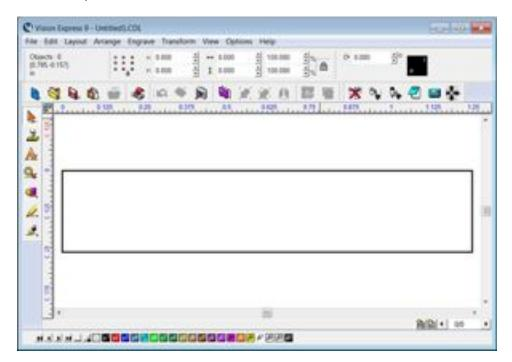
Add text: The Frame Text Compose tool will center and adjust text to fit the plate/engraving area.
