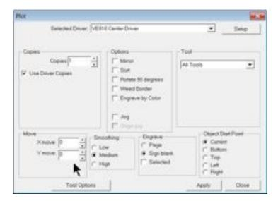
Set the plate size to match the engraving area you determined for your item. In this example, a 1.75" x 0.75" size was entered. Make sure the Selected Driver is the VE810 Center Driver, then click on OK.
