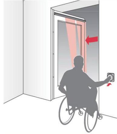
AUTO-IR Presence Sensor and Door Activator 48", length field-adjustable
