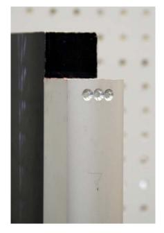
Rod guide holes drilled and counter sunk.
