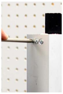
Install rod guide and fasten in place.
