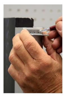
Mark the location for the guide bracket. You can use the factory supplied plastic guide, or upgrade to our steel bracket (LMB-06 square hole or LMB-07 hex Hole).
