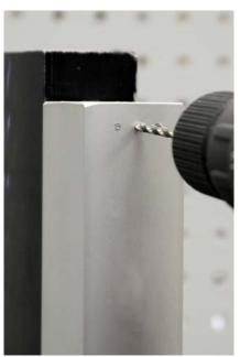
Drill all three marks with a 5/32" drill bit and counter sink for the flat head screws when complete.
