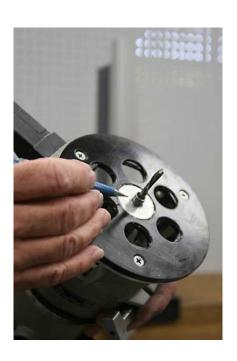
Your router needs to be equipped with a 3/8" outside diameter template guide mounted in its base. Failure to use a template guide will cause the opening being routed to be too large and will damage your HIT-45 template.
