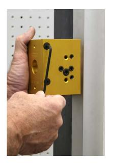
The HIT-32AR drill guide is reversible for both right and left hand doors. The side plates are counter sunk on both sides, just mount the plates on the side needed.
